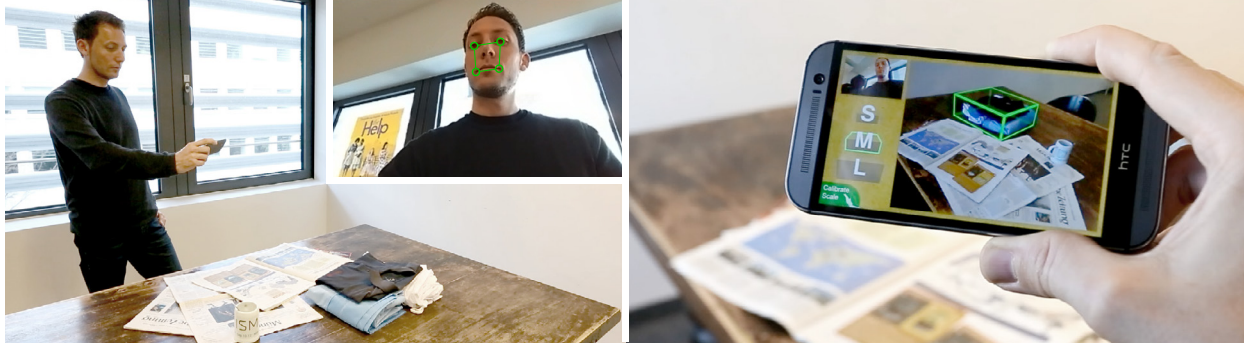
Figure 1: In monocular visual SLAM the structure of a scene as well as the motion of the world-facing camera are only estimated up-to-scale but can be brought to absolute scale by simultaneously capturing and tracking the user’s face in the user-facing camera (left). This enables superimposing virtual objects, e.g. the green wire frame model of a parcel, at absolute scale (right).
