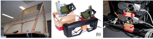
Figure 3: Photographs of our prototype (a); the rear-projection is shuttered using a disassembled pair of shutter glasses (b,c).
