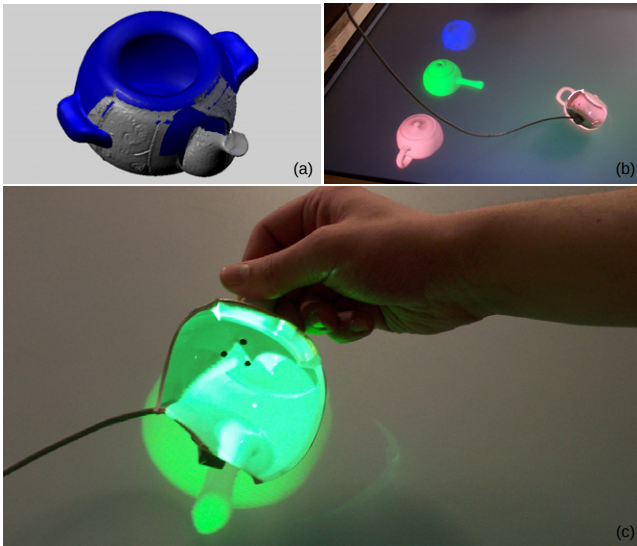
Figure 5: Augmented shards: a scanned shard and possible context (a); choice of different possible contexts to evaluate (b); augmentation of the context of the shard while held in the user's hand (c).
